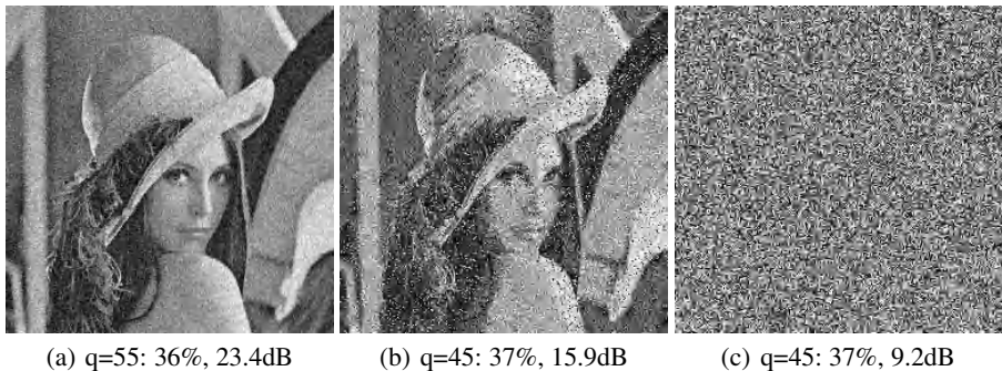
Fig. 2. Catmap with 5 iterations (without extensions and using 3D and diffusion extensions, respectively), keyset 1
